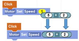
Figure 4. Editing via Dragging and Dropping a Shape Block
