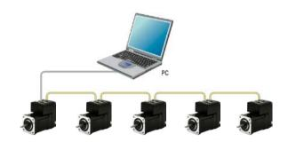
2. Using an integrated high resolution encoder (10000 PPR), the real-time motor position is updated every 50us.
